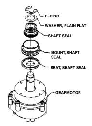
FIGURE 8. SHAFT SEAL 700 AND 1000
